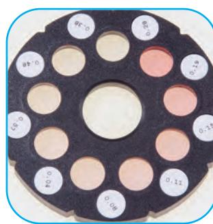
The table on the following pages provides details of the commonly used Lovibond® test discs that are available for water analysis.
