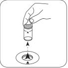
Remove the vial from the sample chamber.
