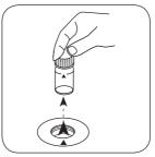
Remove the vial from the sample chamber.
