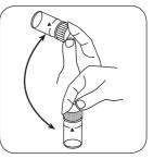
Dissolve tablet(s) by inverting.
