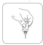
Hold cuvettes vertically and Add 6 drops DPD 1 Buffer Add 2 drops DPD 1 Readd equal drops by pressing Solution. slowly.
