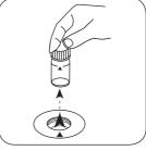
Remove the vial from the sample chamber.
