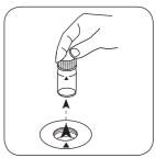
Remove the vial from the sample chamber.
