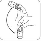
Dissolve tablet(s) by inverting.
