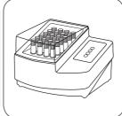
Seal the vials in the preheated thermoreactor for 120 minutes at 100 °C .
