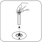
Remove vial from the sample chamber.
