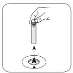
Remove vial from the sample chamber.
