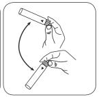
Allow vial(s) to cool to 60°C. Invert several times to mix the contents.
