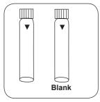
Prepare two reaction vials. Put 2 ml deionised water Mark one as a blank.
