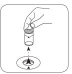
Remove the vial from the sample chamber.
