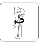
Fill a suitable sample vessel Add IRON LR tablet. with 10 ml sample .
