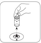
Remove the vial from the sample chamber.
