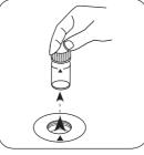
Remove the vial from the sample chamber.
