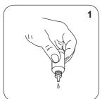
Add 1 drops KS135 (Phenolphthalein Substitute Indikator).
