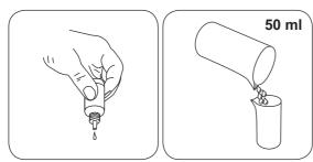
Add **KS 144 (Calcium Hard-**Fill the sample with **deioness Buffer)** drop by drop to the same sample until colouration turns from light pink to red. (Note: make sure to swirl the vial after adding each drop!)
