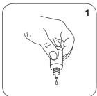
Add 1 drops KS135 (Phenolphthalein Substitute Indikator).
