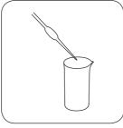
Adjust pH-value of the sam- Fill the sample with deiople with ammonia solution nised water to 100 ml. (10-25 %) to 3-5.
