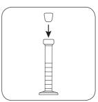
Stopper the mixing cylinder. Swirl around to dissolve the powder.
