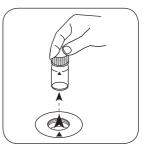
Remove the vial from the sample chamber.
