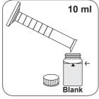
Fill blank with 10 ml prepa- Close vial(s). red sample.
