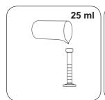
Put 25 ml prepared sample Add Vario (Fe in Mo) Rgt 2 Stopper the mixing cylinder. in 25 ml measuring cylinder. powder pack.
