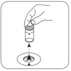
Remove the vial from the sample chamber.
