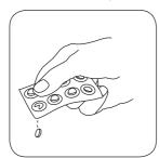
Add PHMB PHOTOMETER Crush tablet(s) by rotating tablet.
