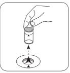
Remove the vial from the sample chamber.
