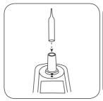
Place the ampoule in the sample chamber.
