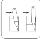
25 ml mark with the sample. in the sampling vessel. Break off the ampoule tip by applying light pressure against the vessel wall. Wait for the ampoule to fill completely.
