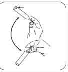
Place a Vacu-vial® ampoule Invert the ampoule several times, allowing the bubble to move from one end to the other. Dry the outside.
