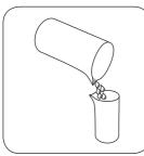
Fill a suitable digestion vessel with **50 ml homoge**nised sample.
