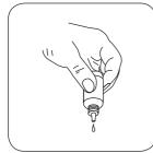
Add KS 144 (Calcium Hard- Fill the sample with deioness Buffer) drop by drop to the same sample until colouration turns from light pink to red. (Note: make sure to swirl the vial after adding each drop!)
