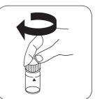
Hold cuvettes vertically and Add **25 drops KS228 (Am**-Close vial(s). add equal drops by pressing **monium Molybdate**). slowly.
