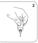
Add 2 drops KS135 (Phenolphthalein Substitute Indikator).
