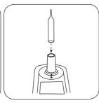
Place the ampoule in the sample chamber.
