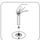
Remove vial from the sample chamber.
