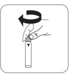
Open digestion vial PO<sub>4</sub>-P Put 5 ml sample in the vial. Close vial(s). Dilution .
