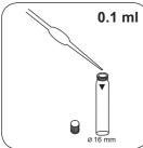
Add 0.1 ml (2 drops) Phos- Close vial(s). phate-101 of the digested sample.
