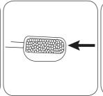
Add a level measuring scoop No. 8 (black) Digestion Reagent.
