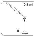
Fill sample vial with 0.5 ml prepared, digested sample.
