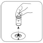
Remove the vial from the sample chamber.
