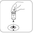
Remove the vial from the sample chamber.
