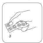
Add **BROMCRESOLPURP-** Crush tablet(s) by rotating LE PHOTOMETER tablet.
