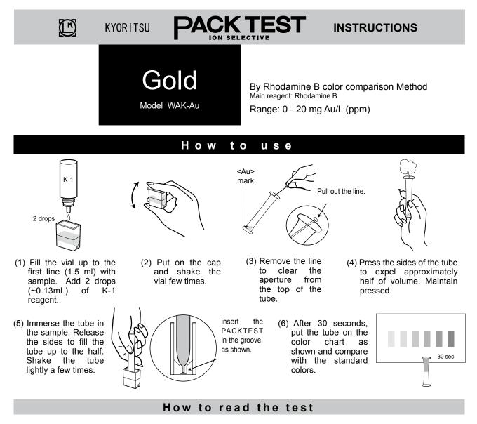
After the reaction time, compare the color of the tube with the standard colors. The nearest color indicates the measured value of the sample. A color between two standard colors indicates a value between the two standard values.
