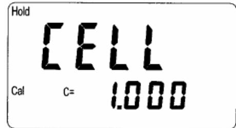
3. When the value of electrode is flashing, pushing up or down button to set the value. Choices of Conductivity, 0.01, 0.05, 1.00, and 10.0, can be selected. After selection, push
