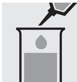
Pipette 0.50 ml of **SO<sub>4</sub>-1** into a test tube.
