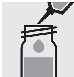
Add 5.0 ml of **sulfuric acid 40 %**, close the cell with the screw cap, and mix.
