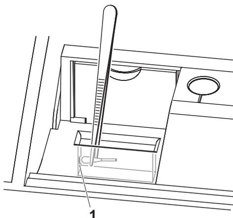
The detector lens is on the front left side of the rectangular cell shaft (pos. 1).
