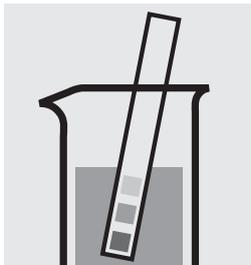
Check the pH of the sample, specified range: pH 6 – 8. If required, add dilute sodium hydroxide solution or sulfuric acid drop by drop to adjust the pH.
