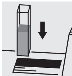
Place the cell into the cell compartment.
