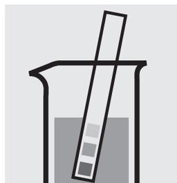
Check the pH of the sample, specified range: pH 2–10. If required, add dilute sodium hydroxide solution or hydrochloric acid drop by drop to adjust the pH.
