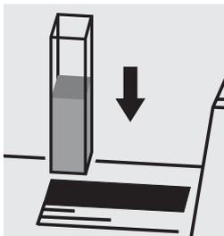
Place the cell into the cell compartment.
