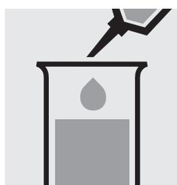
Pipette 5.0 ml of NH<sub>4</sub>-1 into a test tube.
