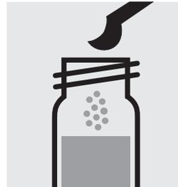
Add 1 level blue microspoon of **Fe-1K**, close the cell with the screw cap.
