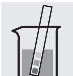
Check the pH of the sample, specified range: pH 0 – 10.
