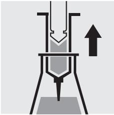
Draw out the liquid to be filtered with the syringe.
