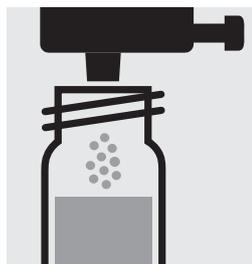
Add 1 dose of **Fe-1K** using the blue dose-metering cap, close the reaction cell with the screw cap.
