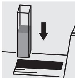
Place the cell into the cell compartment.
