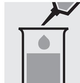
Pipette 10 ml of the pretreated sample into a test tube.
