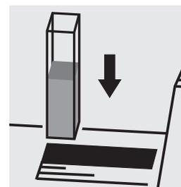
Place the cell into the cell compartment. Select method no. **83**.
