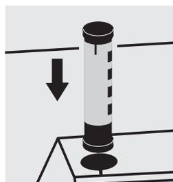
Select method with AutoSelector measuring range 0.10 – 2.00 mg/l F.
