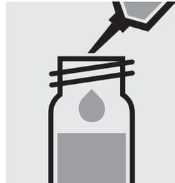
Pipette 5.0 ml of the sample into a test tube with screw cap. **(Important: Do not use test tubes made of glass containing boron!)**
