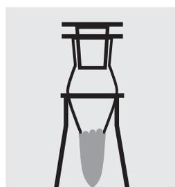
Close the absorption tubes with the glass stoppers, and attach to the top of the Erlenmeyer flasks.
