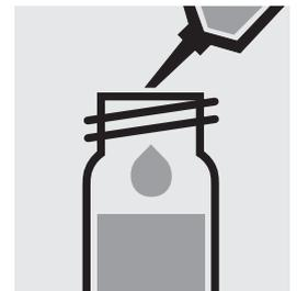
Add 5.0 ml **toluene GR** (Cat.No. 108325) with pipette, close the cell with the screw cap.
