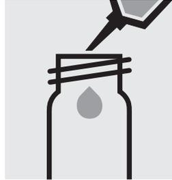
Pipette 5.0 ml of the sample into a reaction cell, close with the screw cap.
