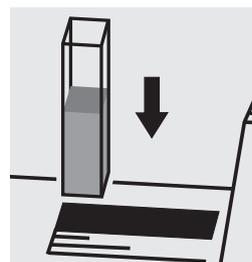
Place the cell into the cell compartment.
