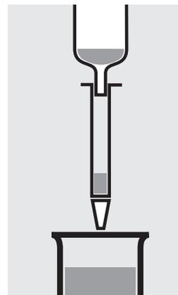
Remove the stopper from the column outlet and run the sample through completely.
