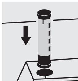
Select method with AutoSelector measuring range 2.0 – 75.0 mg/l NH<sub>4</sub>-N.
