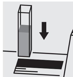
Place the cell into the cell compartment.
