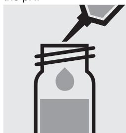
Add 5.0 ml **isoamyl alcohol GR** (Cat.No. 100979) with pipette, close the cell with the screw cap.
