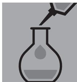
Make the contents of the volumetric flask up to the mark with ethanol, keeping them **protected from light** in the process!
