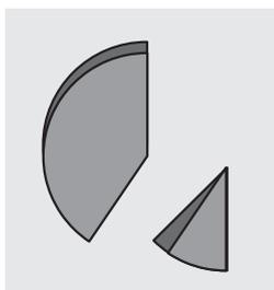
Fold the loaded filter and tear into small pieces.
