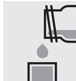
Transfer the solution into a rectangular cell.
