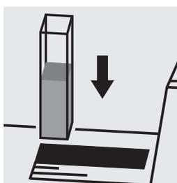
Place the cell into the cell compartment.
