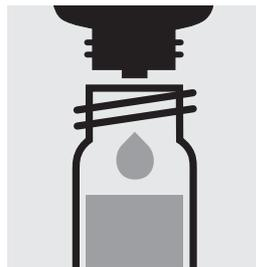
Add to each vessel 3 drops of **Si-2**, close with the screw cap, and mix.
