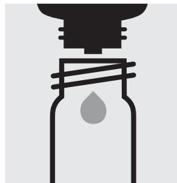
Add 6 drops of **Cr-3K** into a reaction cell, close the cell with the screw cap.
