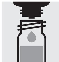
Add 2 drops of **T-1K**, close the cell with the screw cap.
