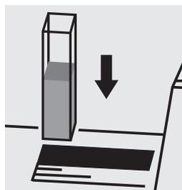
Place the cell into the cell compartment. Select method no. **1195**.
