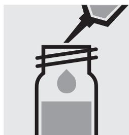
Add 1.0 ml of **OA-4** with pipette, close the cell with the screw cap, and mix.
