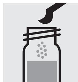
Add 1 level green microspoon of SO<sub>4</sub>-1K, close the cell with the screw cap.
