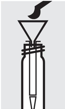
Place the column in an empty cell. Fill 1 level blue microspoon of **AOX-1** into the column using the glass funnel.
