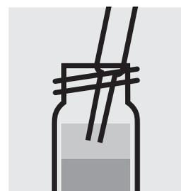
Aspirate the clear upper phase from the tube with pipette.
