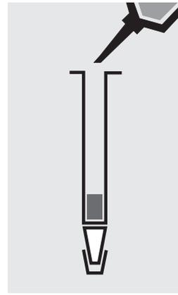
Close the bottom end of the column with the stopper. Apply to the column 1 ml of **AOX-3**. Close the top end of the column with the stopper and swirl to eliminate air bubbles. Remove the stopper on the top end and fill the column to the brim with **AOX-3**.
