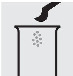
Place 1 level grey micro-spoon of  $\text{SO}_3\text{-1}$  into a dry test tube.
