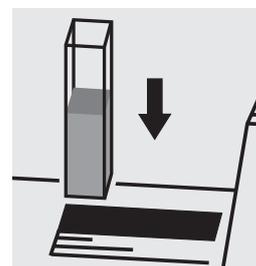
Insert the cell containing the sample into the cell compartment.
