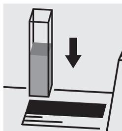
Place the blank cell into the cell compartment.
