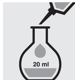
Make up the contents of the volumetric flask to the mark with distilled water (Water for analysis EMSURE<sup>®</sup>, Cat.No. 116754, is recommended) and mix thoroughly: **pretreated sample**.
