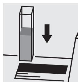
Place the cell into the cell compartment. Select method no. **57**.
