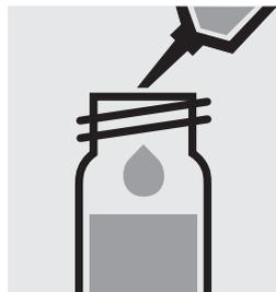
Add 0.50 ml of **OA-4** with pipette, close the cell with the screw cap, and mix.
