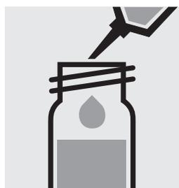
Add 6.0 ml of **Au-4** with pipette, close with the screw cap.
