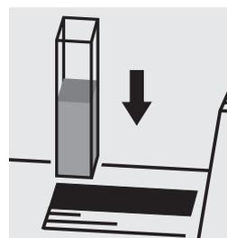
Place the cell into the cell compartment.
