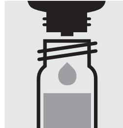
Add 5 drops of **Zn-1**, close the test tube with the screw cap, and mix.
