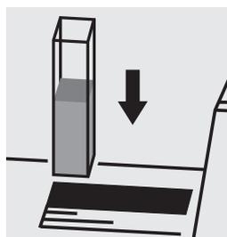
Place the cell into the cell compartment.
