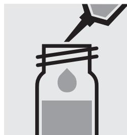
Add 10 ml of the sample with pipette, close with the screw cap, and mix.
