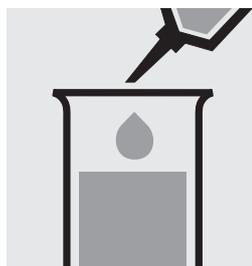
Add 5.0 ml of water and 0.5 ml of the sample with pipette and mix.
