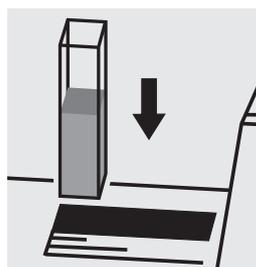
Place the cell into the cell compartment.
