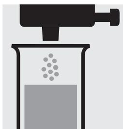
Add 1 dose of **Fe-3** using the blue dose-metering cap and dissolve the solid substance.
