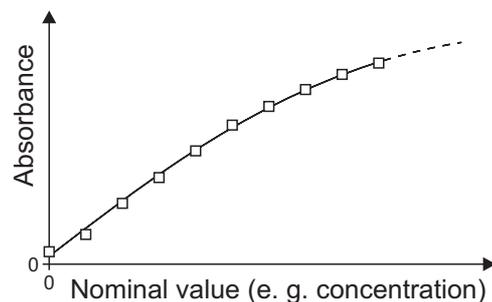
figure 4-4 Example of a parabola calibration function after a 10-point calibration
