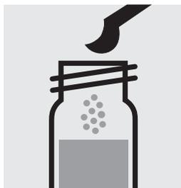
Add 1 level grey micro-spoon of **SO<sub>3</sub>-1K** into a reaction cell, close with the screw cap.
