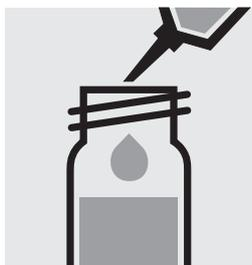
Pipette 0.50 ml of the sample into a reaction cell, **do not mix**.
