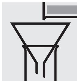
Transfer the residue to a 20-ml volumetric glass using a little distilled water (Water for analysis EMSURE<sup>®</sup>, Cat.No. 116754, is recommended).
