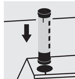
Select method with AutoSelector measuring range 0.5 – 50.0 mg/l Si.
