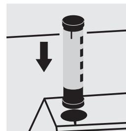
Select method with AutoSelector measuring range 0.025 – 5.00 mg/l.
