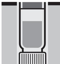
Heat the cell, standing on its head, at 120 °C in the thermoreactor for 2 hours.
