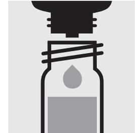
Add 2 drops of **Zn-2**, close the test tube with the screw cap, and mix.
