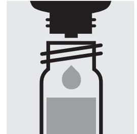
Add 6 drops of **K-1K**, close the cell with the screw cap, and mix.
