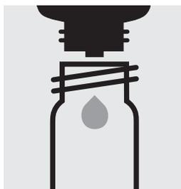
Place 6 drops of **Cl<sub>2</sub>-1** into a round cell.
