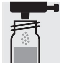
Add 1 dose of **P-2K** using the blue dose-metering cap, close the cell with the screw cap.
