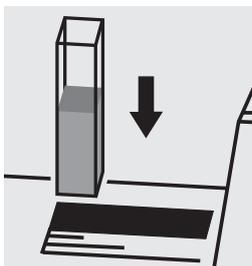
Place the cell into the cell compartment.
