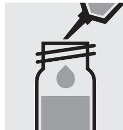
Add 5.0 ml of the **pretreated sample** with pipette, close with the screw cap, and mix.
