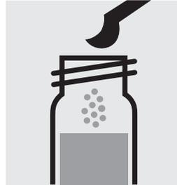
Add 1 level blue micro-spoon of **NO<sub>3</sub>-1K**, **immediately** close the cell tightly with the screw cap. **Caution, foams strongly (eye protection, protective gloves)!**
