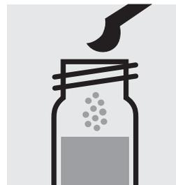
Add 1 level blue micro-spoon of **CN-3K**, close the cell with the screw cap.
