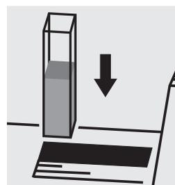
Place the cell into the cell compartment and measure anew.
