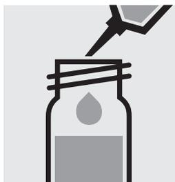
Add 7.0 ml of **pretreated sample** with glass pipette, close the cell with the screw cap, and mix.
