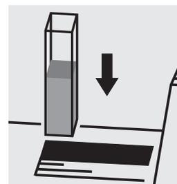
Place the cell into the cell compartment.
