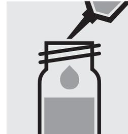
Add 1.5 ml of **B-2** with pipette and close with the screw cap.
