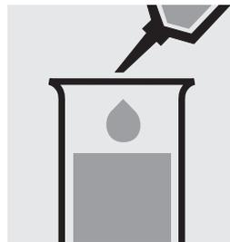
Add **carefully** 0.25 ml of **Mn-4** with pipette and mix **carefully (Foams! Wear eye protection!)**.
