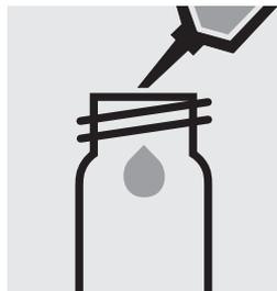
Pipette 5.0 ml of the **pretreated sample** into a reaction cell, close with the screw cap, and dissolve the solid substance.
