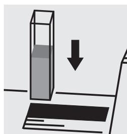
Place the cell into the cell compartment.
