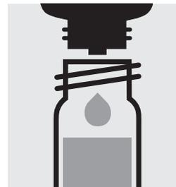
Add 2 drops of **reagent 3**, close the cell with the screw cap, and mix.
