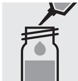
Add 1.0 ml of **Ag-6**, close with the screw cap, and mix.
