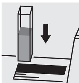
Place the cell into the cell compartment.
