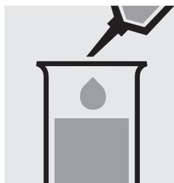
Add 0.20 ml **perchloric acid 70 - 72 % GR** (Cat.No. 100519) with pipette and mix.
