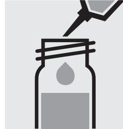
Add 2.0 ml of the sample with pipette, close the cell with the screw cap, and mix. **Caution, cell becomes hot!**
