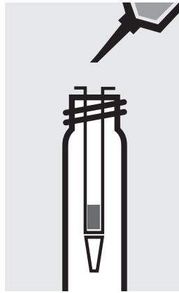
Run 3 separate 1-ml portions of **AOX-2** through the column. Discard the wash solution.
