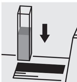
Place the cell into the cell compartment.
