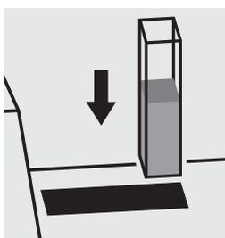
Place the cell into the cell compartment.
