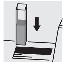
Place the cell into the cell compartment.
