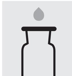
Fill 2 oxygen reaction bottles each with **inoculated nutrient-salt solution** and 2 glass beads to overflowing. Close bubble-free with the slanted ground-glass stoppers.
