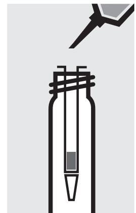
Detach the column from the reservoir. Apply 3 separate 1-ml portions of **AOX-3**. Discard the wash solution.
