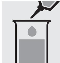
Pipette 4.0 ml of the sample into a test tube.
