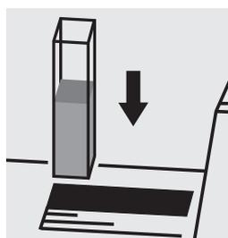
Place the cell containing the sample into the cell compartment.
