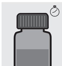
Allow to stand at +4 °C for 0.25 - 24 hours for the extraction to take place.
