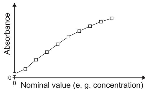
figure 4-3 Example of a polygon line calibration function after a 10-point calibration
