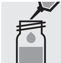
Add 0.50 ml of the sample with pipette, close the cell with the screw cap, and mix.
