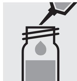
Add 0.50 ml of the sample with pipette, close with the screw cap, and mix.
