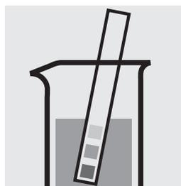
Check the pH of the sample, specified range: pH 2 – 5. If required, add dilute sodium hydroxide solution or sulfuric acid drop by drop to adjust the pH.
