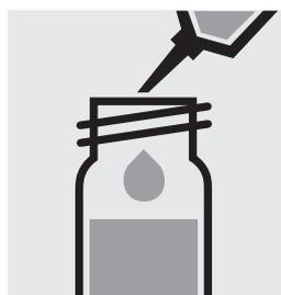
Add 1.0 ml of **OA-4** with pipette, close the cell with the screw cap, and shake vigorously.
