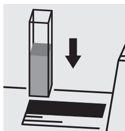
Place the cell into the cell compartment.
