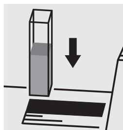
Place the cell into the cell compartment.
