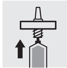
Hold the syringe upright and slowly depress the piston upwards until the membrane-filter is fully wetted free of air bubbles.
