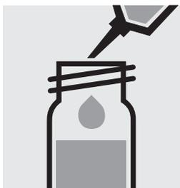
Pipette 0.20 ml of **AOX-1K** into a reaction cell, and mix.
