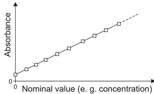
figure 4-2 Example of a linear calibration function after a 10-point calibration
