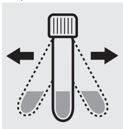
Shake both cells vigorously to dissolve the solid substance.
