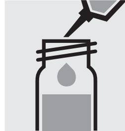
Add 0.50 ml of **T-1K** with pipette and close with the screw cap.
