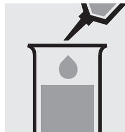
Add 1.5 ml of **reagent 2** with pipette and mix.
