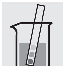
Check the pH of the sample, specified range: pH 3 – 9. If required, add dilute sodium hydroxide solution or hydrochloric acid drop by drop to adjust the pH.
