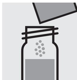
Add 1 powder pack of **Molybdenum HR1**, close with the screw cap, and dissolve the solid substance.
