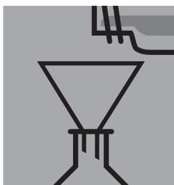
Filter the extract **protected from light** through a paper filter ("Blauband") into a volumetric flask (for DIN 38412: 100 ml). Rinse the filter with a small portion of ethanol.
