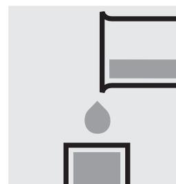
Transfer the clear **lower** phase into a cell.
