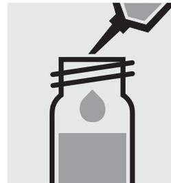
Add 0.20 ml of **Oxyscav 2** with pipette, close with the screw cap, and mix.
