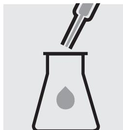
Pipette with glass pipette 20 ml of the sample into a 300-ml Erlenmeyer flask with NS 29/32.
