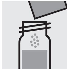
Add 1 powder pack of **Oxyscav 1** and close with the screw cap.
