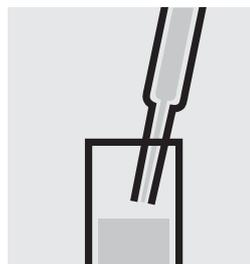
Transfer the solution into a rectangular cell.
