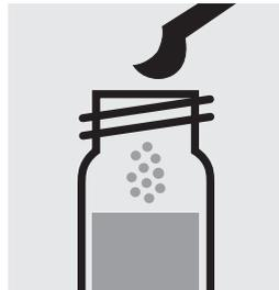
Add 2 level green microspoons of **AOX-6**, close the cell with the screw cap, and mix.
