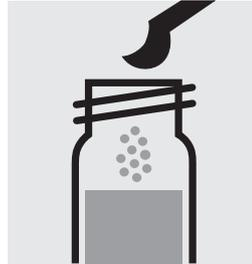
Add 1 level grey microspoon of **Ph-1K**, close the cell with the screw cap.
