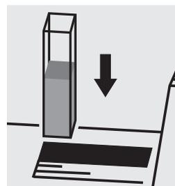
Place the cell into the cell compartment.
