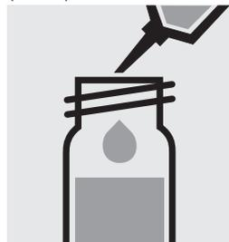
Add to each vessel 0.50 ml of **Si-3** with pipette, close with the screw cap, and mix.
