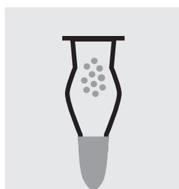
Fill 6 - 7 g each of **Sodalime with indicator** (Cat. No. 106733) into two absorption tubes (Cat. No. 115955).
