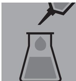
To differentiate the chlorophyll-a content and for the determination of the phaeophytin-a content, acidify a portion of the extract with **hydrochloric acid 2 mol/l Titripur®** (Cat. No. 109063) (0.3 ml per 100 ml of extract).
