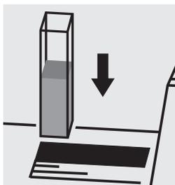
Place the cell into the cell compartment.
