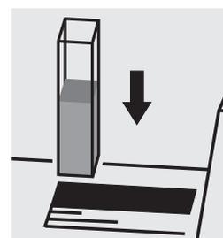
Place the cell into the cell compartment. Select method no. **133**.
