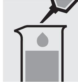
Add 1 ml of **hydrochloric acid 1 mol/l Titripur®** (Cat. No. 109057) with pipette and mix.
