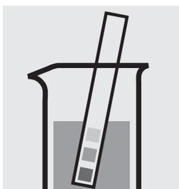
Check the pH of the sample, specified range: pH 2–10.
