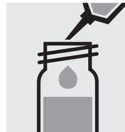
Add 5.0 ml of **OA-5** with pipette, close the cell with the screw cap, and shake vigorously.
