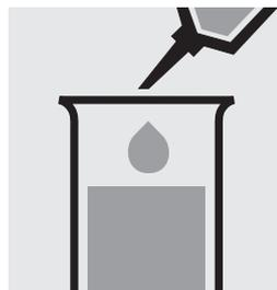
Add 1.2 ml of **PO<sub>4</sub>-1** with pipette and mix.
