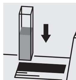
Place the cell into the cell compartment.
