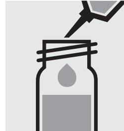
Pipette 10 ml of distilled water into a second reaction cell, close with the screw cap, and mix. (Blank)
