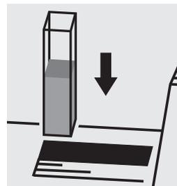
Place the cell into the cell compartment.
