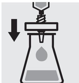
Filter sample solution through a membrane filter with 0.45  $\mu\text{m}$  pore size.
