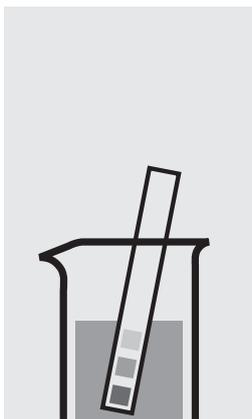
Check the pH of the sample, specified range: pH 6 – 7. If required, add dilute sodium hydroxide solution or nitric acid drop by drop to adjust the pH.
