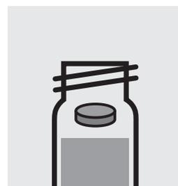
Add 1 **reagent tablet Cyanuric Acid**, crush with stirring rod, and close with the screw cap.
