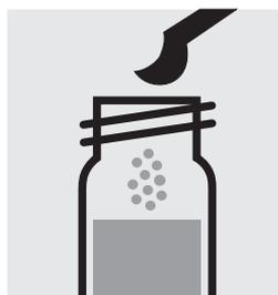
Add 1 level blue micro-spoon of Cl<sub>2</sub>-1, close with the screw cap.
