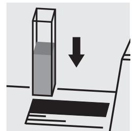
Place the cell into the cell compartment.
