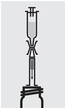
Fill the 10-ml syringe with 10 ml of reagent **AOX-5** and attach the syringe with the column outlet using the connector. Place the top end of the column on an empty cell and rinse the charcoal filling of the column into an empty 16-mm cell.
