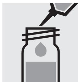
Add 1.0 ml of **OA-5** with pipette, close the cell with the screw cap, and shake vigorously.
