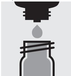
Add 5 drops of O<sub>2</sub>-2K, close the cell with the screw cap, and shake for 10 seconds.
