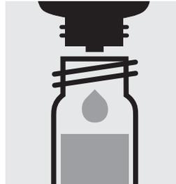
Add 2 drops of **Mn-1K**, close the cell with the screw cap, and mix.
