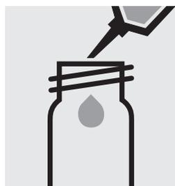
Add 9.0 ml of distilled water (Water for analysis EMSURE®, Cat.No. 116754, is recommended) with pipette.
