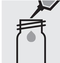
Pipette 1.0 ml of **B-1K** into a reaction cell, close with the screw cap, and mix.
