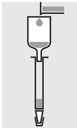
Fill 100 ml of the sample and 6 drops of **AOX-4** into the reservoir.
