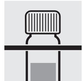
Replace the cell in the rack for complete cooling to room temperature. **Very important!**
