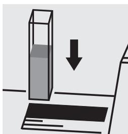
Place the cell into the cell compartment.
