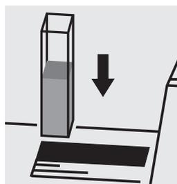
Place the cell into the cell compartment.
