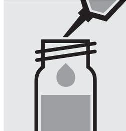
Add 10 ml of the sample with pipette, close the cell with the screw cap.
