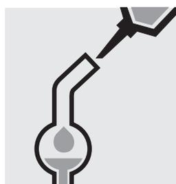
Pipette 5.0 ml of **As-5** into the absorption tube.
