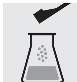
Add 3 level red dosing spoons of **As-7**. **Immediately** attach the absorption tube to the Erlenmeyer flask.
