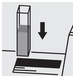
Place the cell into the cell compartment.
