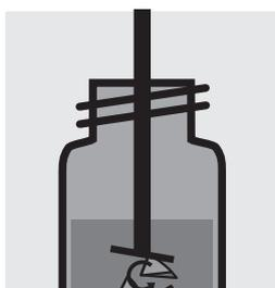
Disintegrate the filter in the homogenizer.
