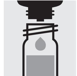
Add 3 drops of **Mn-2K**, close the cell with the screw cap, and mix.
