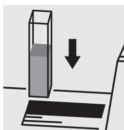
Place the cell into the cell compartment.
