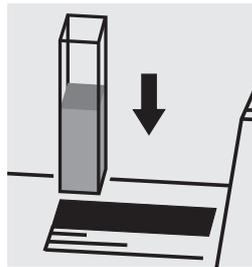
Place the cell into the cell compartment.
