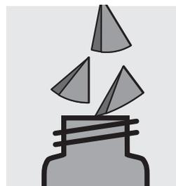
Place the pieces of the filter in an extraction vessel (e.g. 100-ml amber glass bottle).
