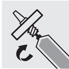
Screw the syringe tightly into the front side of the membrane-filter attachment.
