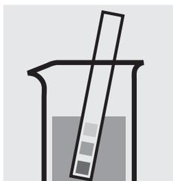
Check the pH of the sample, specified range: pH 3 – 8.
