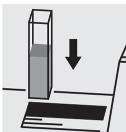
Place the cell into the cell compartment.
