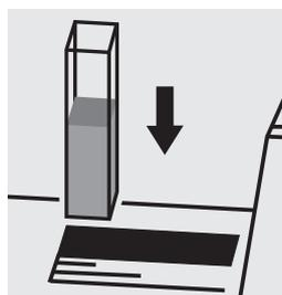
Place the cell into the cell compartment.
