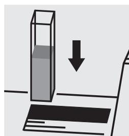
Place the cell into the cell compartment.
