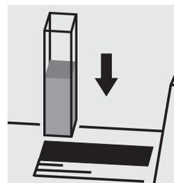
Place the cell into the cell compartment. Select method no. **130**.
