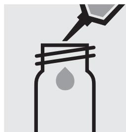
Pipette 5.0 ml of the sample into an empty test tube (e. g. flat-bottomed tubes cells, Cat.No. 114902).
