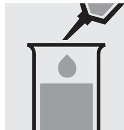
Add to the second tube 10 ml of distilled water (Water for analysis EMSURE®, Cat.No. 116754, is recommended) with pipette and mix. (Blank cell)
