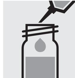
Add 1.0 ml of **B-1** with pipette, close with the screw cap, and mix.
