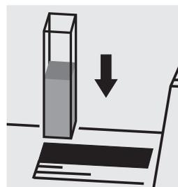
Place the cell into the cell compartment.
