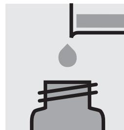
Add approx. 30 ml of boiling **ethanol** (w = 90 %) and allow to cool to room temperature.
