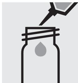
Pipette 5.0 ml of the **pretreated sample** into an empty round cell (Empty cells, Cat.No. 114724).
