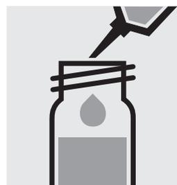
Add **5.0 ml of distilled water** (Water for analysis EMSURE<sup>®</sup>, Cat.No. 116754, is recommended) with pipette, close with the screw cap, and mix.
