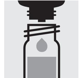
Add 2 drops of **reagent 1**, close the cell with the screw cap, and mix.
