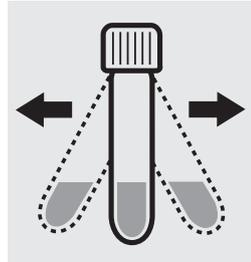
Shake the cell vigorously to dissolve the solid substance and leave to stand for **1 minute**.
