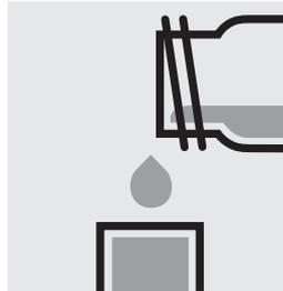
Transfer the solution (when possible without sediment) into a corresponding rectangular cell.
