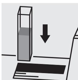
Place the cell into the cell compartment.
