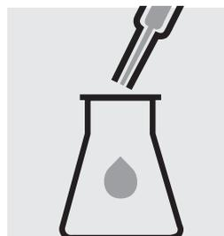
Pipette with glass pipette 20 ml of distilled water (Water for chromatography LiChrosolv®, Cat.No. 115333, is recommended) into a second 300-ml Erlenmeyer flask with NS 29/32.
