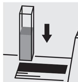
Place the cell into the cell compartment.
