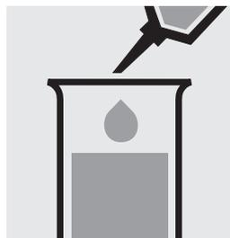
Pipette 0.50 ml of **Pb-1** into a test tube.
