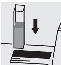
Place the cell into the cell compartment.
