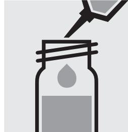
**Carefully** pipette 3.0 ml of the sample into a reaction cell, close tightly with the screw cap, and mix vigorously. **Caution, the cell becomes hot!**
