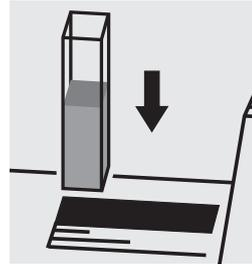
Place the cell into the cell compartment.
