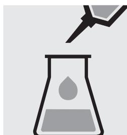
Add 1.0 ml of **As-6** with pipette to the solution in the Erlenmeyer flask and mix.
