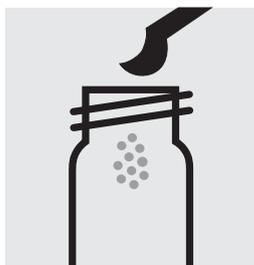
Add 2 level blue microspoons of NO<sub>2</sub>-1K into a reaction cell.
