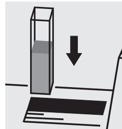
Place the cell into the cell compartment.
