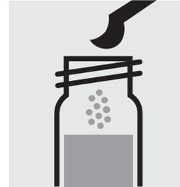
Add 1 level green microspoon of **Cd-2K**, close the cell with the screw cap.
