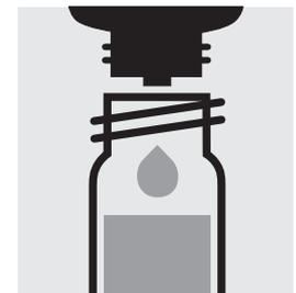
Add 15 drops of **B-5**, close with the screw cap, and mix.
