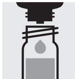
Add 3 drops of **Ag-3**, close with the screw cap, and mix.
