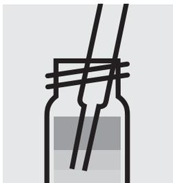
Aspirate 0.5 ml of the clear lower phase from the tube with pipette.
