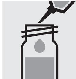
Pipette 5.0 ml of the sample into a reaction cell, close with the screw cap, and mix.
