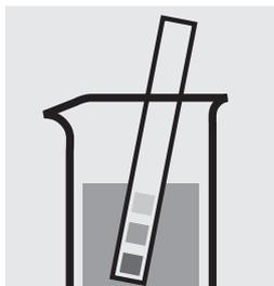
Check the pH of the sample, specified range: pH 4–9. If required, add dilute sodium hydroxide solution or sulfuric acid drop by drop to adjust the pH.
