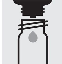
Add 6 drops of **Cr-3K** into a reaction cell, close with the screw cap.
