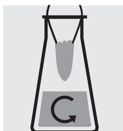
Stir at 250 rpm for 2 h at room temperature: depleted sample / depleted blank
