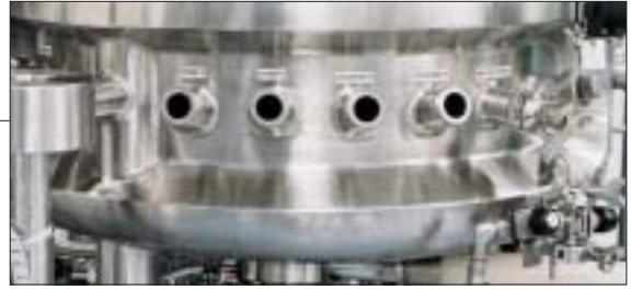
Dual pH electrode and D.O. sensor side ports on a B. Braun Biotech 400 liter bioreactor.
