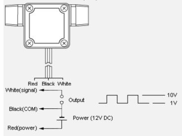
When the 12V DC power '+' pole is covered to red, and the '-' pole is connected to black, a 'high=10V, low 1V' rectangluar wave occur between white and black.
