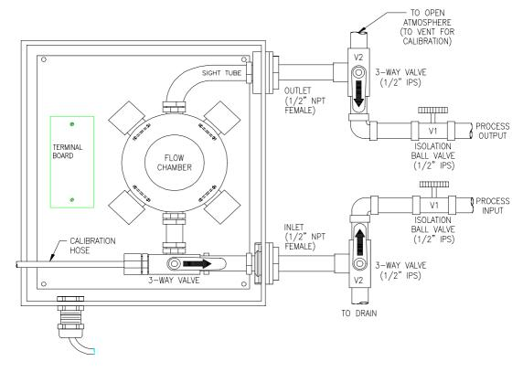
FIGURE 2-1 Recommended Closed-loop Sensor Piping Arrangement
