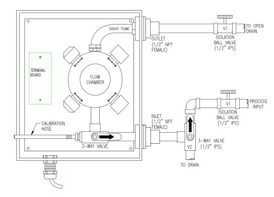
FIGURE 2-2 Recommended Sample Bypass Line Sensor Piping Arrangement
