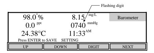
Using the [UP], [DOWN] and [DIGIT] soft-keys, enter the true local barometric pressure. This corresponds to a reading from a mercury barometer. Do **NOT** use the pressure reported by the weather bureau. Weather bureaus correct pressures to sea level.
