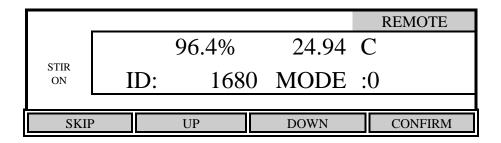
The Remote mode is used in conjunction with YSI 5910 *BOD Analyst* software to greatly reduce the labor required for processing BODs and calculating BOD values.
