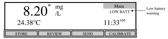
When this happens, replace the batteries with 4 fresh alkaline C-size batteries as soon as possible.
