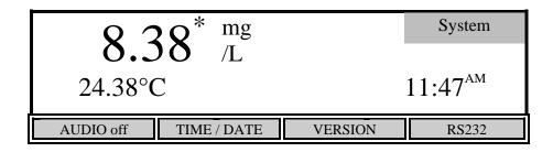
The [AUDIO on/off] soft-key allows setting the beeper on or off. The key toggles between an [AUDIO off] soft-key and an [AUDIO on] soft-key. The present state of the beeper would be the OPPOSITE of the function shown on the soft-key. If the beeper is currently on, the soft-key shows "AUDIO off"; i.e., your alternate choice.
