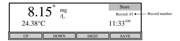
The Store menu is used to control the storing of data. The current record number is shown in the display on the right side.
