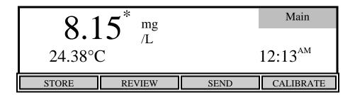
The bottom row of the display shows the functions of the four soft-keys used during Main mode. Main mode is used to make measurements, store or review readings and send the current readings to a computer or serial printer.
