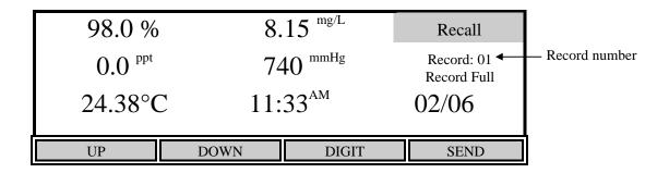
The Recall menu is used to recall or send data that was previously stored. The current record number is shown on the right side of the display.
