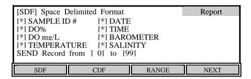
The display lists the parameters that can be included in the output string at the RS232 serial port, the default set has everything selected for inclusion.
