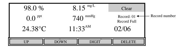
The Clear menu is used to delete data that was previously stored. The current record number is shown in the display on the right side.
