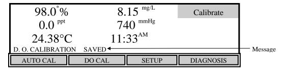
9. Press [MODE] to return to the Main mode. The instrument is now calibrated and ready to measure dissolved oxygen and temperature. See 7.1 Main Mode, Making Measurements.
