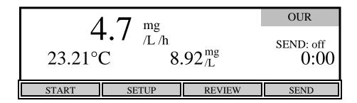
Press [SETUP] to change the OUR parameters. The following screen shows the default parameters.
