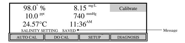
NOTE: For accurate DO readings, the salinity setting MUST match the salinity of each sample measured.
