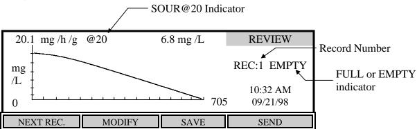
Press the [NEXT REC.] soft-key to change the record number to find an empty slot, or pick a slot to overwrite (you cannot delete results, you must overwright). Press the [SAVE] soft-key to save the current test data into that slot. Once you have saved the data you can press the [MODIFY] soft-key to change the parameters of the test.
