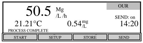
NOTE: The DO and temperature readings do not stop updating on the screen.
