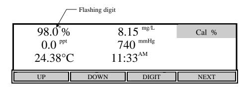
8. Make sure that the display readings are stable, then enter the calibration value in percent saturation, using the [UP], [DOWN] and [DIGIT] soft-keys. See *Appendix A - Oxygen Solubility Table* and *Appendix B - Pressures and Altitudes* for manual calibration data.
