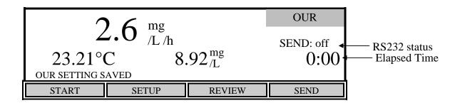
Once the parameters have been set, you are ready to begin. Place the probe in the prepared sample and make certain no air bubbles are trapped, then turn on the stirring and wait a few seconds for the temperature readings to stabilize.
