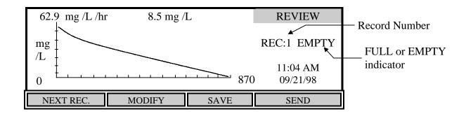
Press the [NEXT REC.] soft-key to change the record number to find an empty slot, or pick a slot to overwrite (you cannot delete records, you must overwright). Press the [SAVE] soft-key to save the current test data into that slot. Once you have saved the data you can press the [MODIFY] soft-key to change some parameters of the test.
