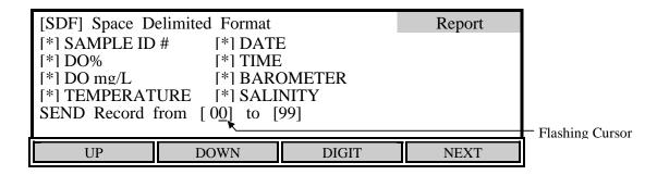
This menu allows specifying a specific range of memory locations for the report. The default range is 00 - 99 and empty locations will not be sent to a computer or serial printer.
