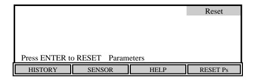
Press [ENTER] to confirm. All parameters, including calibration values, will be reset. If you do NOT wish to reset the parameters, press [MODE], instead of [ENTER], to return to the Diagnosis menu.
