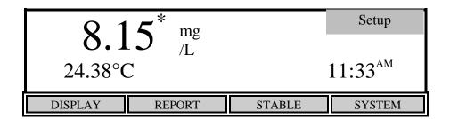
These four selections are used to change the instrument setup.
