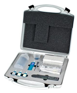
The Bresle Test is one of the most popular tests for extracting and measuring the salt contamination on blast-cleaned substrates.
