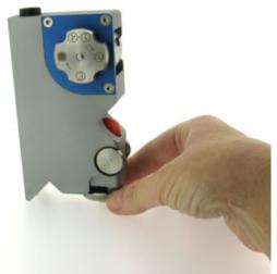
5. Read the graduation-scale and multiply the divisions with the D factor engraved on the SuperPIG.
