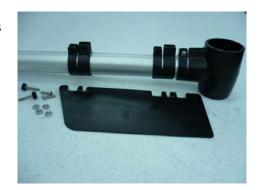
Install the fin as shown with the alignment tab on the fin inserted into the slot on the propeller housing at the end of the flow probe pole.
