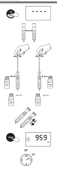
Remove the cap of vial A. Use the 3 mL plastic pipette to transfer the upper layer (organic phase) into a cuvet.
