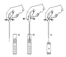
Repeat step a), b) and c) until all the organic solvent is transferred. Ensure that at least 1/3 of the cuvet is filled with organic solvent, otherwise erroneous results will be obtained. Notes:
