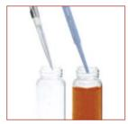
Step 2 Add reagent in the cuvet then insert it in the instrument and note the reading.
