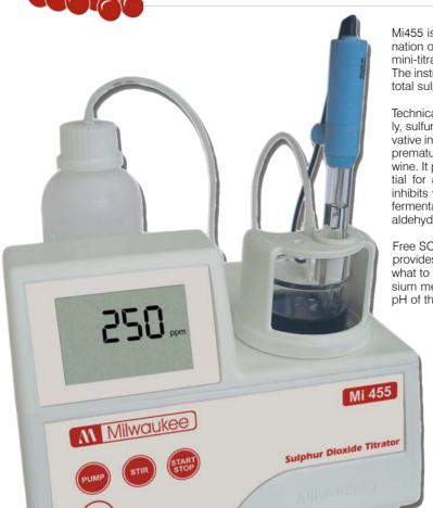
Mi455 is a user-friendly microprocessor-based mini-titrator for the determination of free and total sulphur dioxide in the process of wine making. This mini-titrator will give you direct readings with a range of 0 to 400 ppm. The instrument comes with a pre-programmed analysis method for free and total sulphur dioxide measurements on wine sample.
