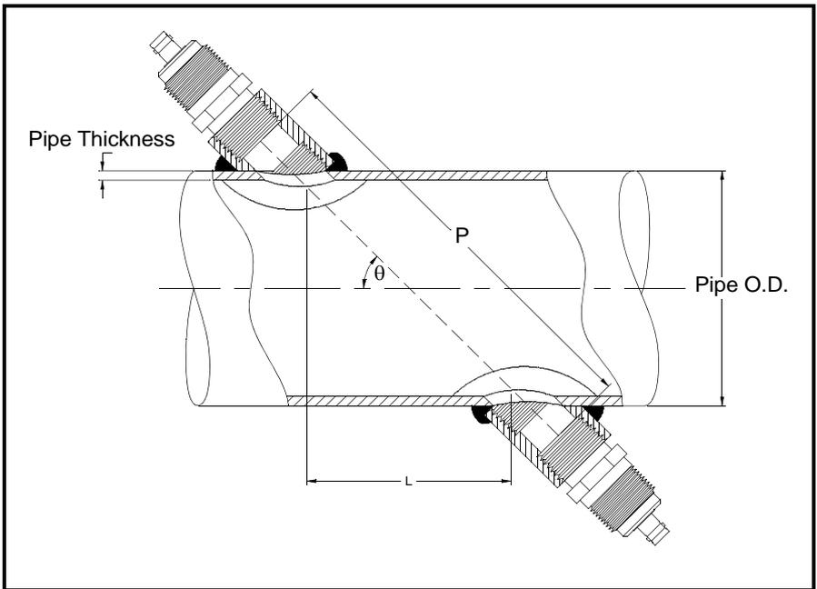
Figure 154: Top View of 180° Transducer Installation
