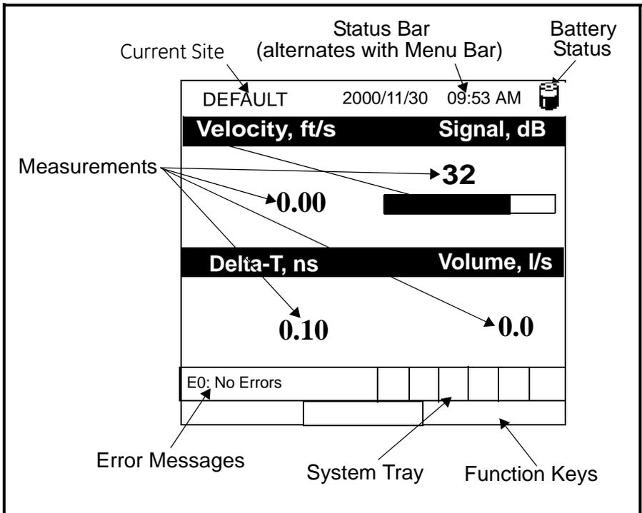
Figure 6: PT878 Screen in Operate Mode
