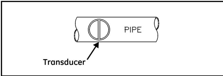
Figure 157: Proper Alignment of Transducers for Cylindrical Surfaces
