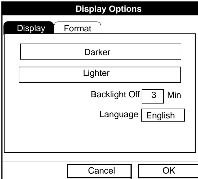
Figure 80: Display Tab in the Display Options Window
