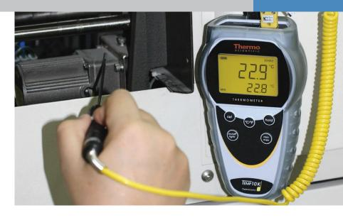
Rugged and easy to use, the Thermo Scientific Temp 10 Series features a large, backlit dual-line LCD, giving you clear, accurate readings of measured and min/max temperature, even in dark environments. Ergonomically designed to fit your palm perfectly, the Temp 10 series offers maximum hands-free convenience with our exclusive three-way hands-free kit\*.
