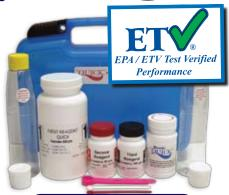
Arsenic Quick™ Kit Part No. 481396 This kit can also be used for soil Arsenic Testing.
