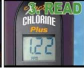
Fill built-in cell and zero meter
