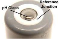
Junction In the center of the measuring surface is the pH sensitive flat glass surface. This surface is surrounded by the flat
