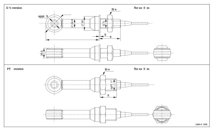
Dimensions: ersions with G ¾ thread top and PT thread bottom
