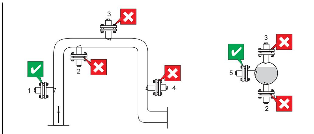
Orientation and installation positions (with adapter CUA120-A/B resp. retractable assembly CUA451)
