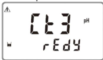
When measuring the second standard buffer's mV value, the sign
