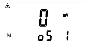
8.2.3 The display shows the previous calibration SLP (Slope) value. Pressing
