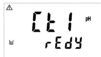
2. The display will show mV value while being calibrated. After the value becomes stable, the display will show the first pH value of calibration. Then, it will enter the second calibration (Ct2).
