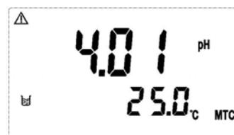
3. Clean the electrode completely, and put it into the second buffer solution. Then, press
