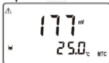
When measuring the second standard buffer's mV value, the sign
