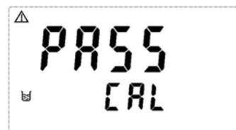
7. The display will automatically show the oS1 (zero-point mV) Value. Press
