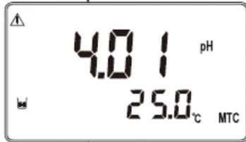
PC-3100 to finish the Tech buffer two point calibration.
