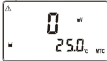
When measuring standard buffer's mV value, the sign
