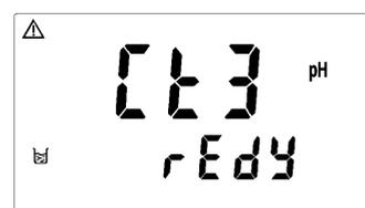
5. Clean the electrode completely, and put it into the third buffer solution. Then, press
