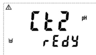
4. The display will show the mV value while being calibrated. After the value becomes stable, the display will show the second pH value of calibration automatically. Then, then it will enter the third-point calibration (Ct3).
