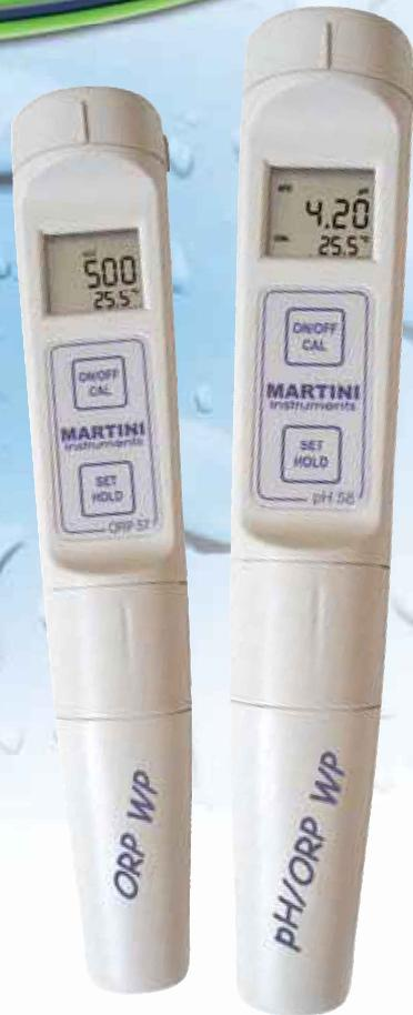
Combination waterproof testers with advanced functions also include the new model pH58 for simultaneous pH and ORP measurements and temperature, which is continuously displayed on the dual level LCD. It shows readings in an extended range from -2.00 to 16.00 pH or 1000 m and simultaneously shows temperature from -5.0 to 105.0C or 23 to 221F.
