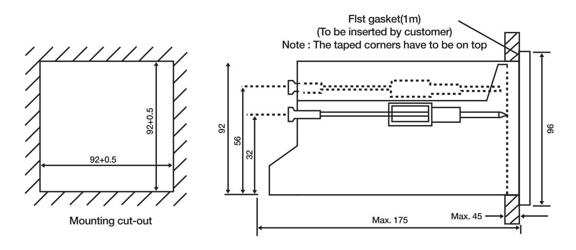
The field-tested control panel housing is 96 x 96 mm; with protection class IP 54 (front)
