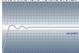
Rapid alignment of the temperature with the set value with minimum oscillations
