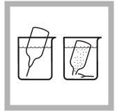
2. Prepare the blank: Pour at least 40 mL of ozone-free water in a 50-mL beaker. Fill an Indigo Ozone Reagent AccuVac Ampul with the ozone-free water. Keep the tip immersed while the Ampul fills fully.
